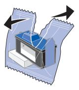
2 Remove the tape and packaging from the cartridges.
